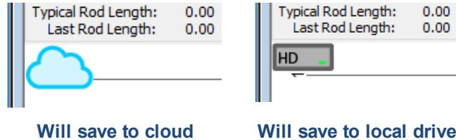
To save to a different location, select **File > Save As....** In the dialog box, enter a **DataLog Name** and then click **Local** or **Cloud** as appropriate. To save to the cloud, Cloud Manager must be open and you must be logged in; after the job has finished uploading, it will appear in CM.
