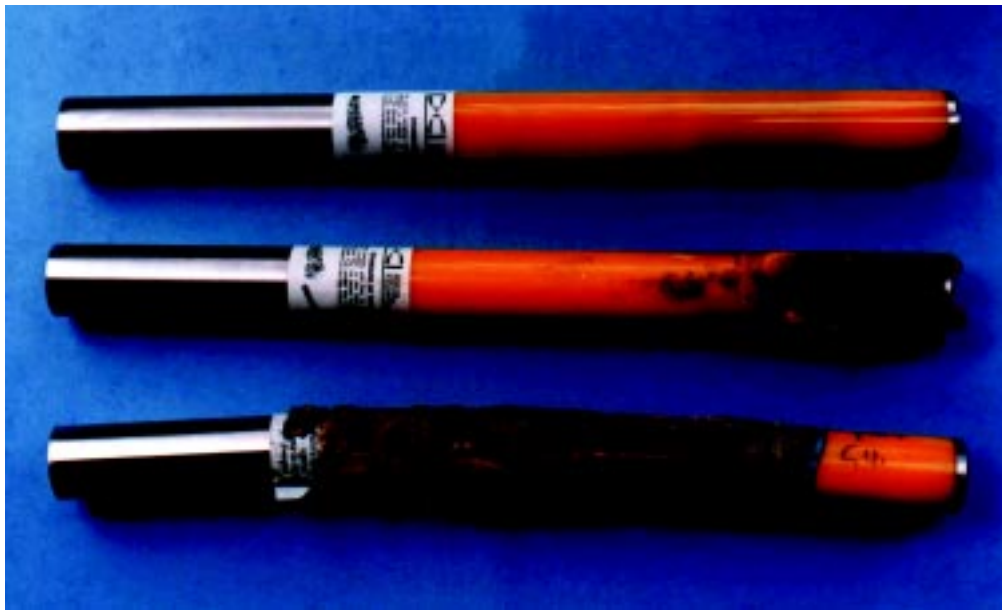
The good, the bad, and the ugly—Transmitters can be severely damaged by overheating.
