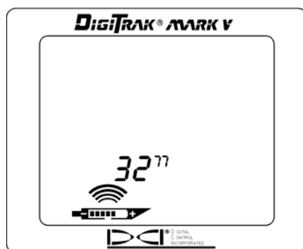
Receiver Frequency Display After Releasing Held Trigger
