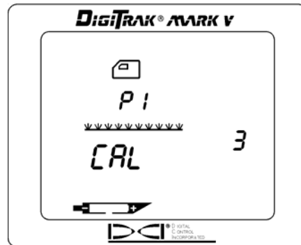
2-Point Calibration Screen – First Point
