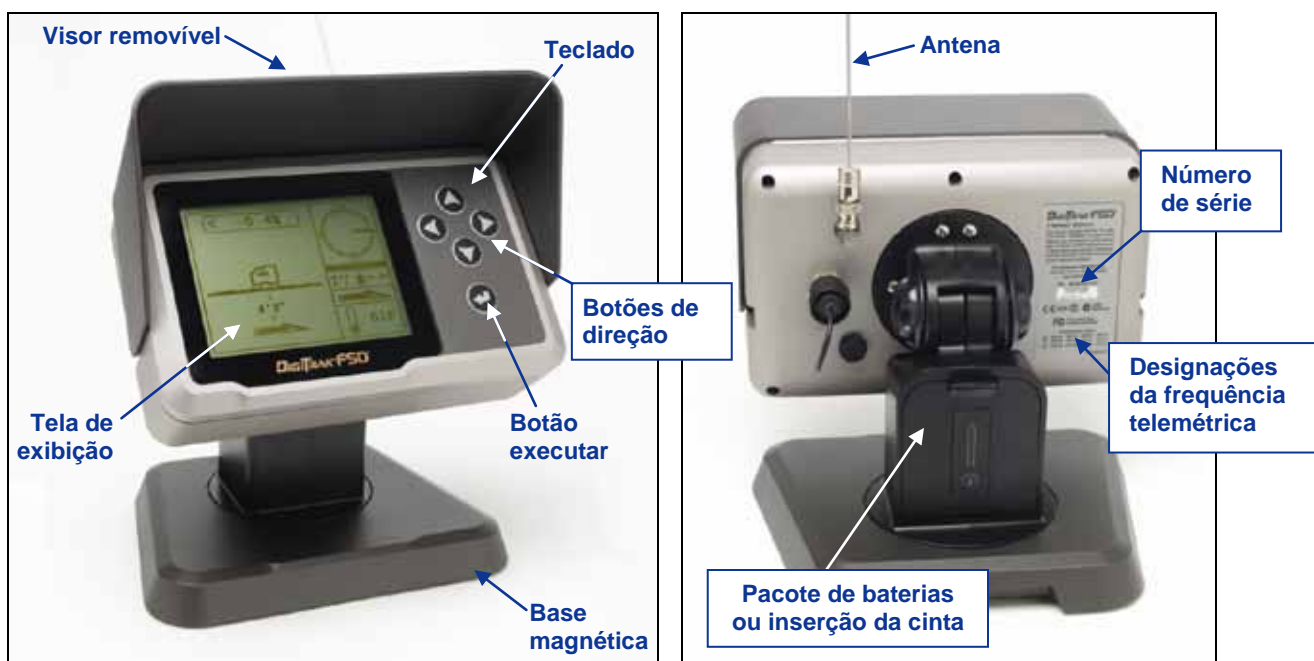
Frente e traseira do visor F Series DigiTrak (FSD)
