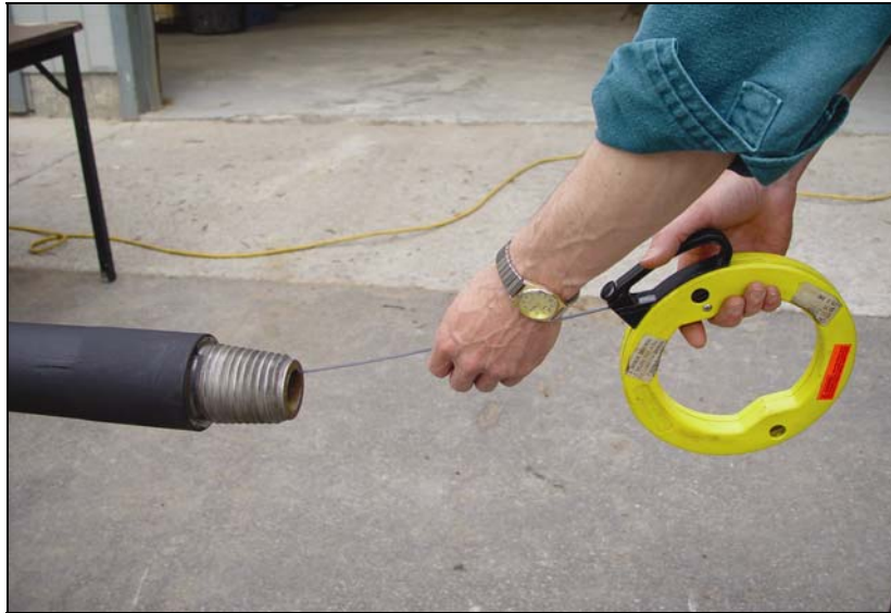
Pushing Fish Tape into Rod from Pin End to Box End
