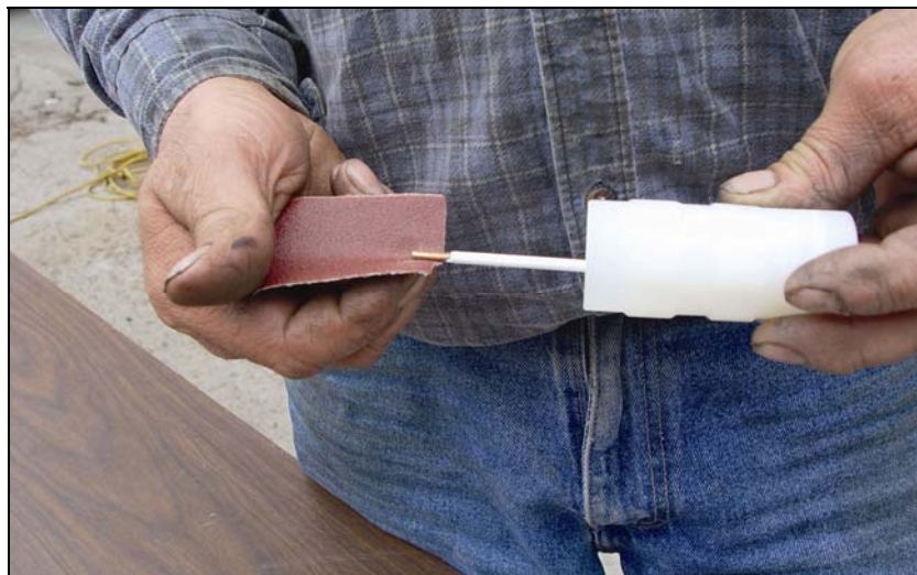
Emery Cloth to Remove Oxidation and Sharp Edges from the Rod on the Pin End
