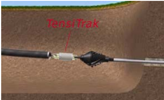
Figure 7. The TensiTrak monitoring system
