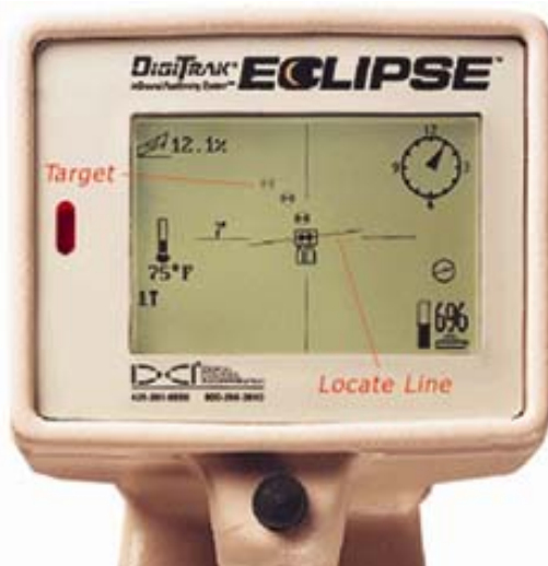
Figure 4. Eclipse receiver locating screen
